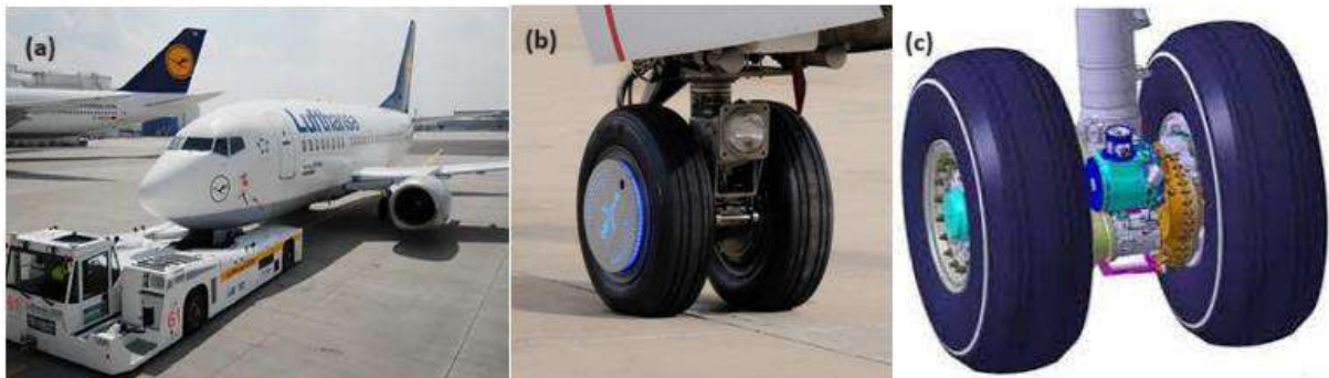
Şekil-1 (a) TaxiBot (Taxibot, 2023), (b) WheelTug (Brookfieldav, 2023), (c) EGTS (Arts et Metiers, 2023)
