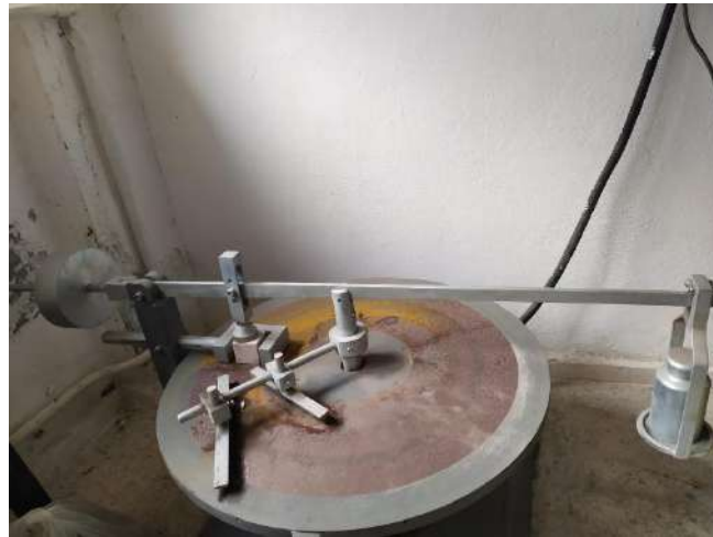
Figure 3. Representation of the Böhme abrasion device
