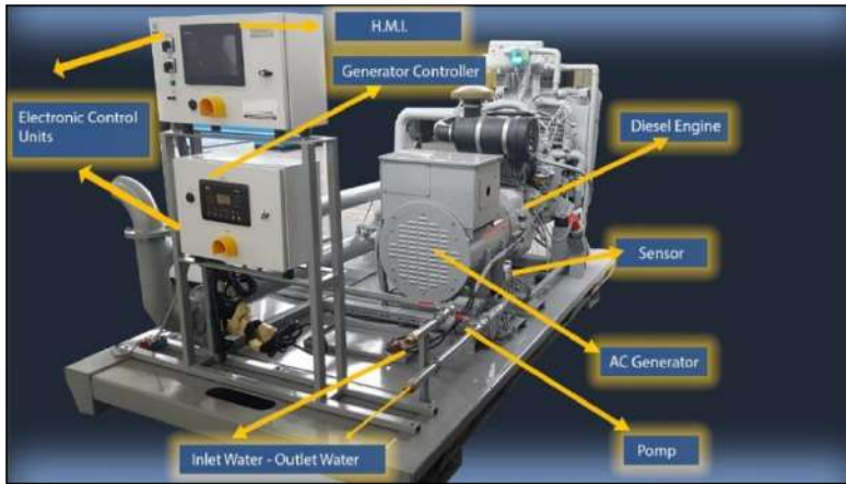
Figure 9: Micro Cogeneration System.
