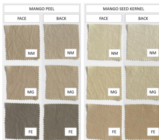
Figure 2. Warp (100% cotton) dominant face sides and weft (100% lyocell) dominant back sides of fabrics dyed with mango peel and seed kernel extracts; no mordant (NM), mordanted with magnesium sulphate (MG) and mordanted with ferrous sulphate (FE)
