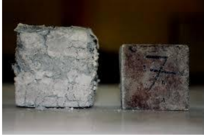
Figure 1. Deterioration of concrete due to sulphate effect (Baradan et al., 2010)
