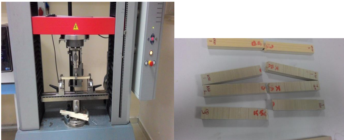
Fig 4. The bending test device and the post-test image
