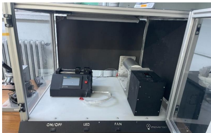
Figure 2. Electrospinning device used in the study
