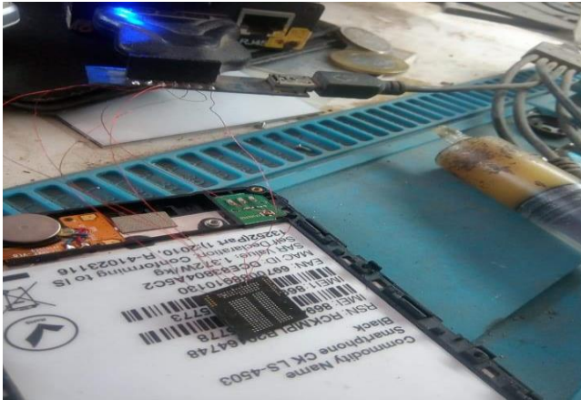
Fig 3: Connectivity of eMMC and PC Through EasyJTAG
