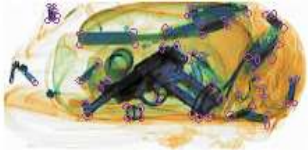
Figure 4: An example x-ray image with the object corners highlighted as purple circles (Akçay, Breckon, Devereux, & Kundegorski, 2016).
