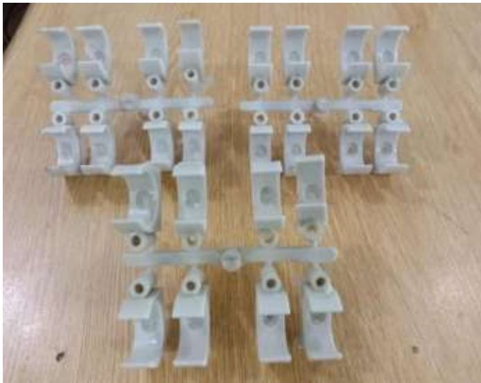
PRODUCT AFTER EXPERIMENTATION OF DIE PVC PIPE CLIPS
