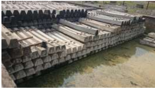
Fig-5 Post-tensioned sleepers
