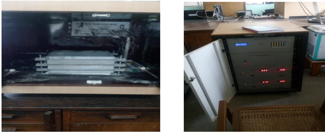
Fig-5 Guarded hot plate method
