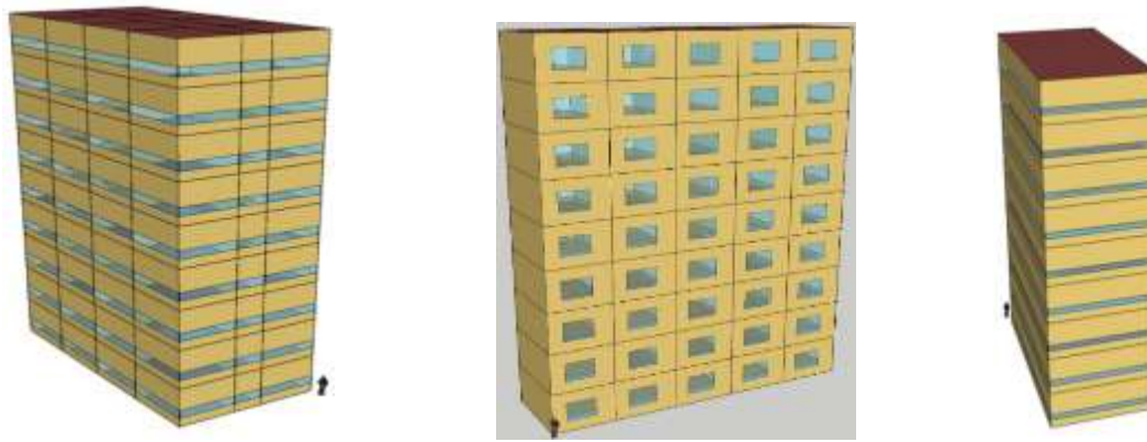
Plate I. Prototypes of double-banked, single-banked and open-plan midrise offices (from left to right).
