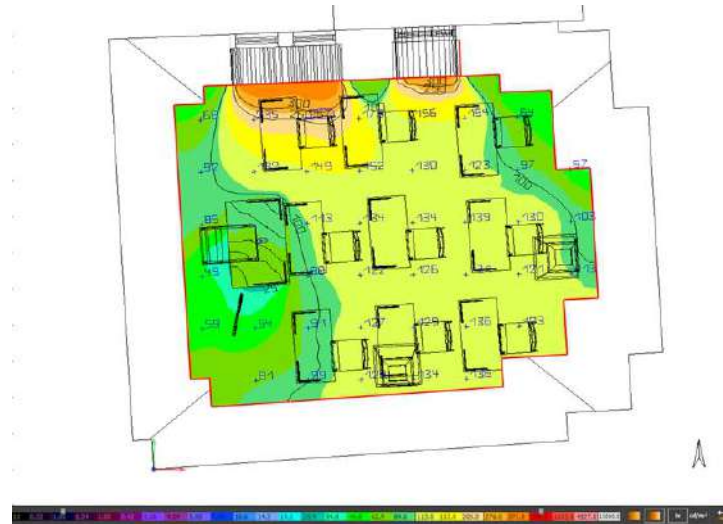
Figure 8: Contour diagram for classroom “2” optimization by adding two skylights (93.8lux to 122 lux)
