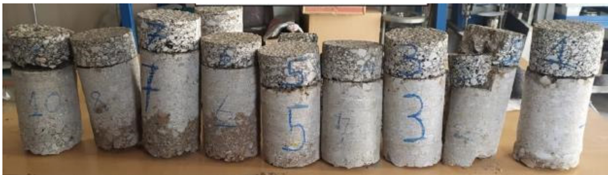
Figure 9. Core samples taken from the pavement (2022)
